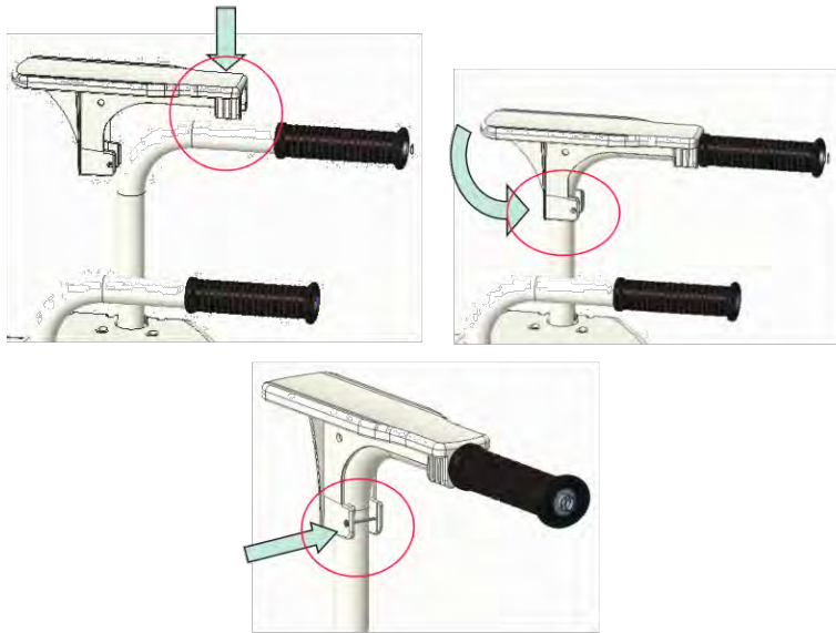
Figure 6 Installation of arm support
